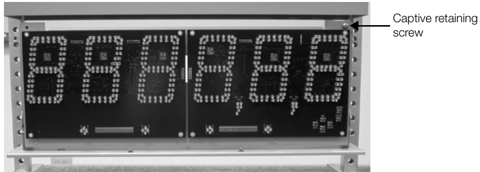
Figure 2-6. LED Primary and Secondary Display Boards (7-Segment Display)
