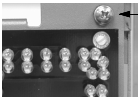
Figure 2-3. Retaining Screw Location
